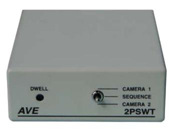
The 2PSWT is a basic two position homing and sequencing video switcher. The front panel controls consist of a three position toggle switch for homing to either camera one or two or setting the dwell time via a recessed pot in the front panel. The dwell time can be set from approximately two seconds to one minute. The 2PSWT is powered by a 9-12VDC and is supplied with a UL appoved wall transformer.
