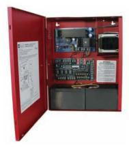
The AL602ULADA, AL802ULADA and AL1002ULADA are extremely cost effective voltage regulated remote NAC Power Extenders. They may be connected to any 12 or 24 volt Fire Alarm Control Panel (FACP). Primary applications include Notification Appliance Circuit (NAC) expansion (supports ADA requirements) and will provide auxiliary power to support system accessories.
